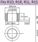
1/2" BSPP female fitting, 304L stainless steel, for welding on 27.6mm hole
