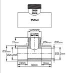
34" BSPP male PVC Tee for bonding on DN25 PVC pipe
