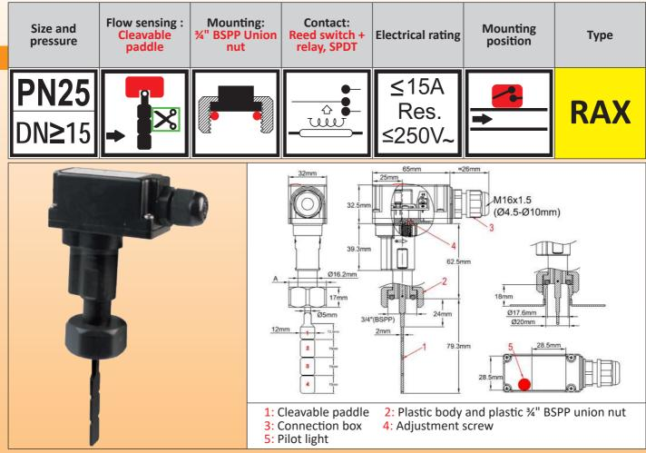
Main uses: General application in flow detection. Recommended mounting position is on horizontal pipes, but can be mounted in any position. For water flow detection on dia 15 to 100mm water pipes. The built-in relay with SPDT contact can be used on resistive loads up to 15A 250V. The pilot light shows the contact position.
