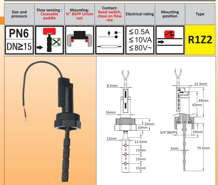
**Main uses:** <u>Large quantities applications</u> in flow detection in low voltage electronic circuits. The most economical model. Recommended mounting position is on horizontal pipes. Can be mounted in any position with a small drift in the calibration because of the paddle weight. Can be used on **15 to 100mm diameter** water pipes.
