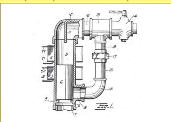
1930 Walker magnetic flow sensor for water heater: the metal piston (6) moves between two magnetic coils (3 and 4) US Patent 1962795.
