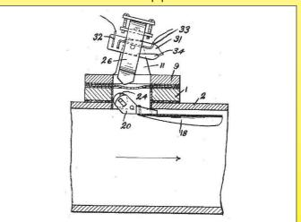
In 1931, the first paddle switch with a magnetic action is invented by Louis E. Richmond (US Patent 1888737). A paddle with a metallic roller actuates a balanced magnet with a mercury switch located outside.
