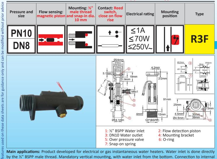
Main applications: Product developed for electrical or gas instantaneous water heaters. Water inlet is done directly by the ½" BSPP male thread. Mandatory vertical mounting, with water inlet from the bottom. Connection to internal copper piping DN10 with quick coupling. Built-in overpressure valve.
