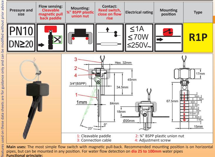
Main uses: The most simple flow switch with magnetic pull-back. Recommended mounting position is on horizontal pipes, but can be mounted in any position. For water flow detection on dia 25 to 100mm water pipes **Functional principle:**
