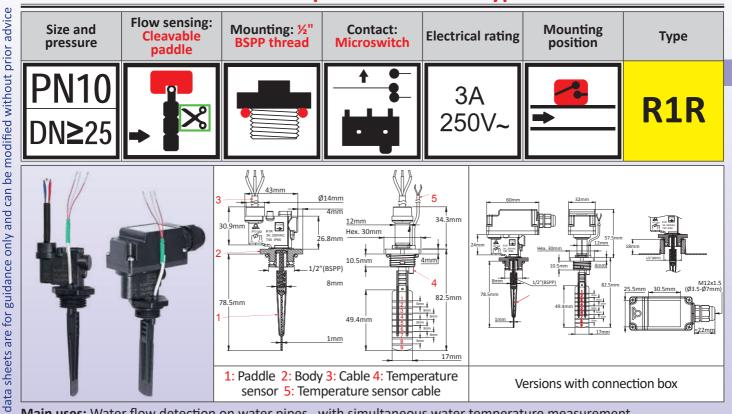
Main uses: Water flow detection on water pipes, with simultaneous water temperature measurement Functional principle: Balanced paddle, perpendicular to the main flow, actuating a micro-switch. Flexible elastomeric gasket between paddle and electric switch. Temperature measurement is made by a plastic pocket located under the 1/2" thread
