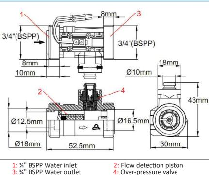
Main applications: Product developed for electrical or gas instantaneous water heaters. ¾" BSPP male water inlet and outlet. Mandatory vertical mounting, with water inlet from the bottom. Built-in over-pressure valve.
