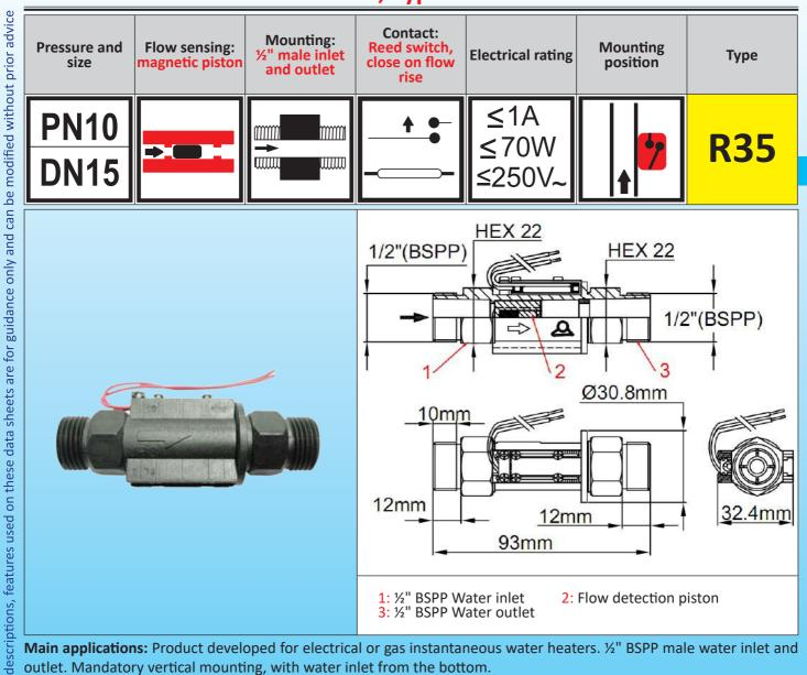
Main applications: Product developed for electrical or gas instantaneous water heaters. ½" BSPP male water inlet and outlet. Mandatory vertical mounting, with water inlet from the bottom.
