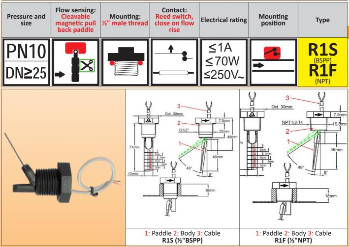
**Main uses:** The most simple flow switch with magnetic pull-back. Recommended mounting position is on horizontal pipes, but can be mounted in any position. For water flow detection on **dia. 25 to 63mm** water pipes **Functional principle:**
