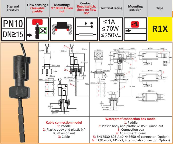
**Main uses:** General application in flow detection. Recommended mounting position is on horizontal pipes, but can be mounted in any position. For water flow detection on **dia 15 to 100mm** water pipes **Functional principle:**
