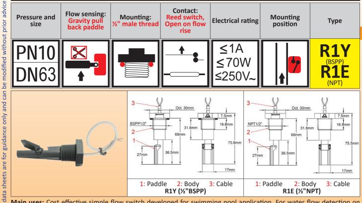
**Main uses:** Cost effective simple flow switch developed for swimming pool application. For water flow detection on **vertical dia 63mm** water pipes, upstream flow
