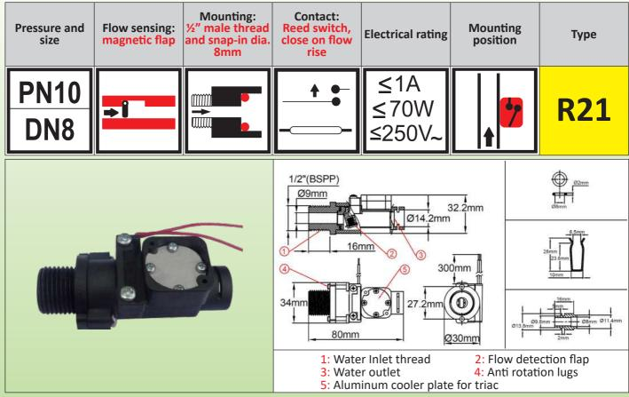
Main applications: Product developed for miniature instantaneous water heaters for showers. The mobile flap system provides compactness. Water inlet is done directly by the ½" BSPP male thread. Mandatory vertical mounting, with water inlet from the bottom. Connection to internal copper piping DN8 and DN10 with quick coupling. A built in aluminum heat exchanger, in contact with the cold water input is provided to cool a triac.
