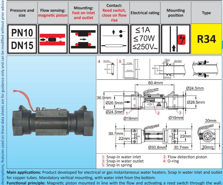
Main applications: Product developed for electrical or gas instantaneous water heaters. Snap in water inlet and outlet for copper tubes. Mandatory vertical mounting, with water inlet from the bottom.
